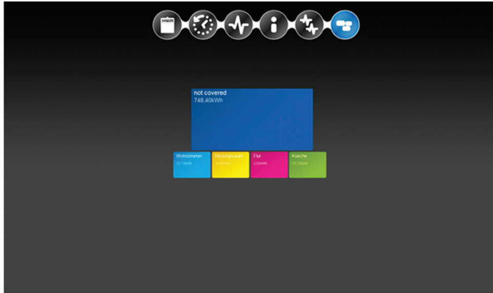
Comparative Tag Cloud: The tag cloud shows sums of consumption of SmartPlugs grouped by user-generated tags.
