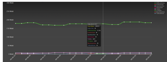
Real-Time Power Information: This screen provides real-time visualization of the current power usage, measured by the SmartPlugs and the SmartPowerMeter . The visualization can be filtered according to tag groups.
